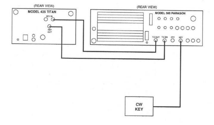
FIGURE 5-7. QSK HOOK-UP WITH TITAN AMPLIFIER
