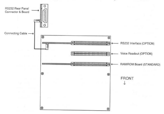
FIGURE 5-3. OPTIONS INSTALLATION DIAGRAM
