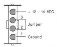
FIGURE 1-1. POWER SUPPLY CONNECTIONS
